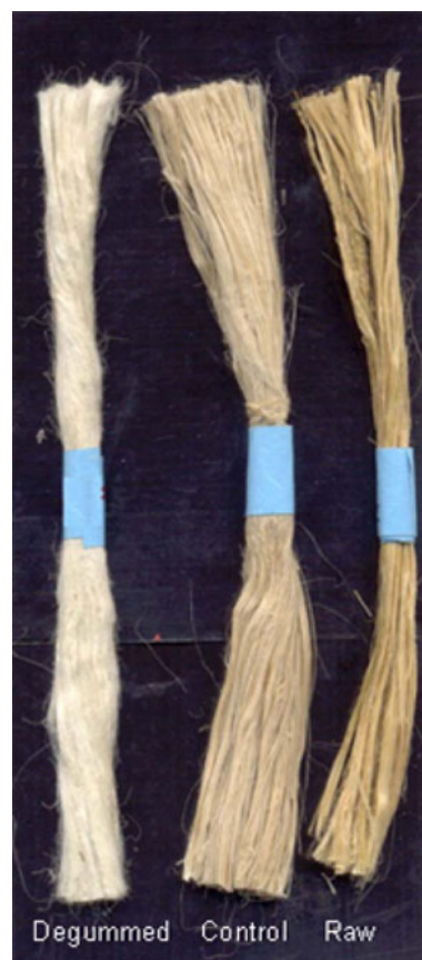
Fig. 1 a Degumming of ramie fibre using purified DKS1 pectate lyase
